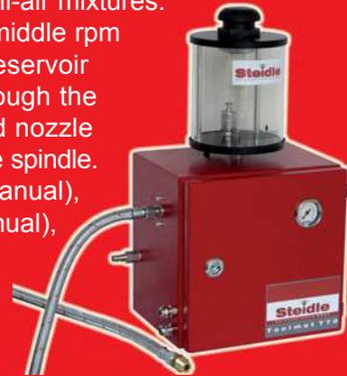
With Toolmat® T70 the proven piston pumps provide for an exactly selectable flow rate. The spray grade can be determined via the spray air. The saturation of the mixture can be adjusted via the casing air. In the Vario3 and Vario7 versions, 3 or 7 pre-settable oil quantities can be selected.
