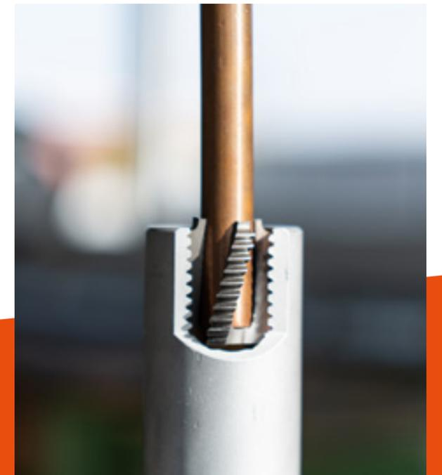
Vaporisation releases the cutting edges and allows them to be easily removed. The electrode does not come into contact with the workpiece, meaning that the thread remains undamaged. The company's standard choice of drilling emulsion is used as the coolant.
