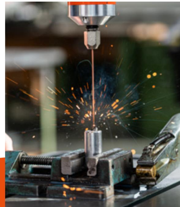
The hollow copper electrode is clamped in the oscillating head. It is smaller in diameter than the broken-off tool. During the erosion process, the core of the broken-off tool is vaporised by spark discharge.
